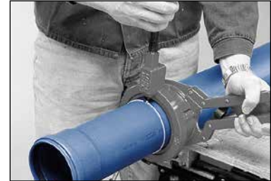
Cutting to length with a cutting and chamfering tool (FIGURE 16)
